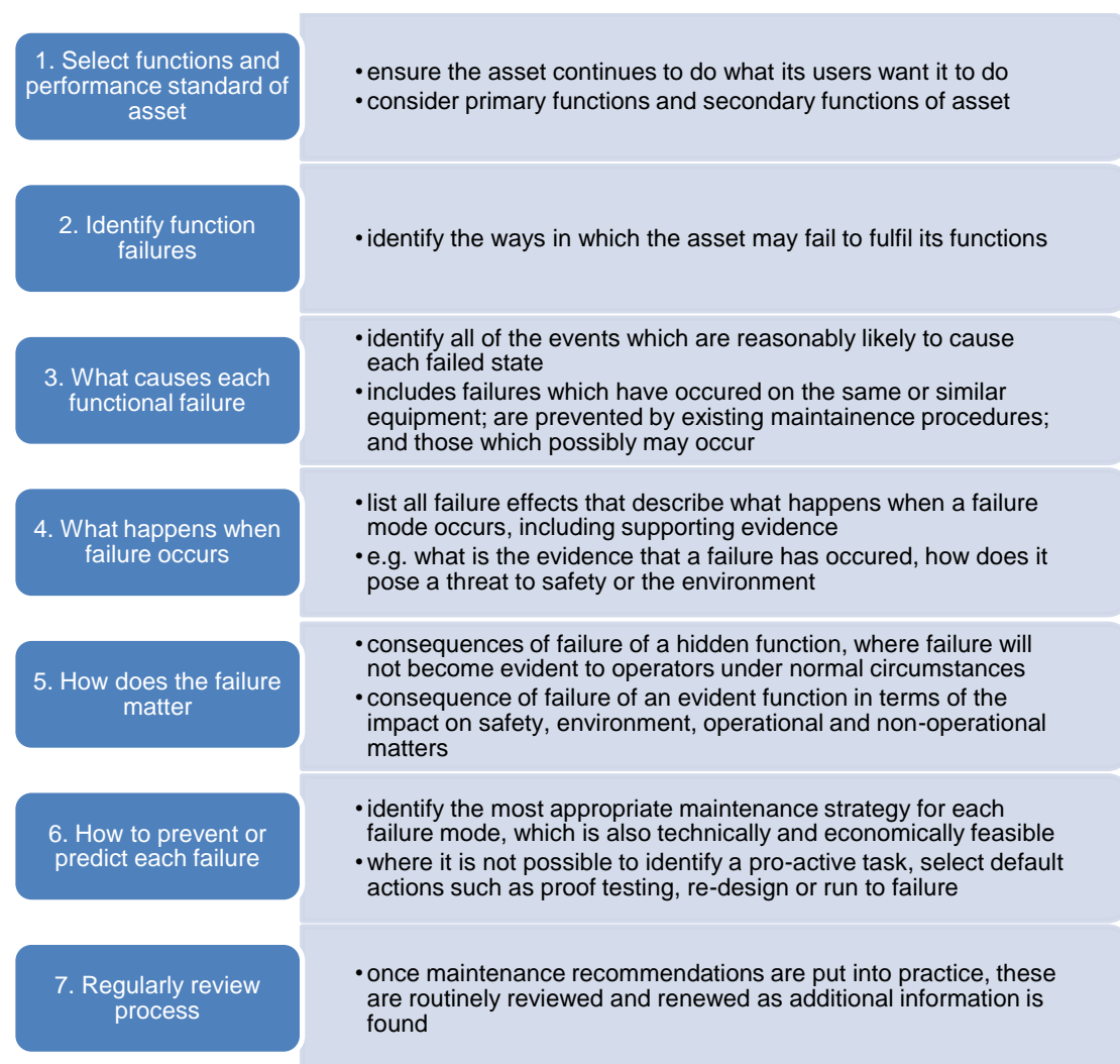
Figure 13.1 Steps in the RCM process to develop a maintenance strategy
